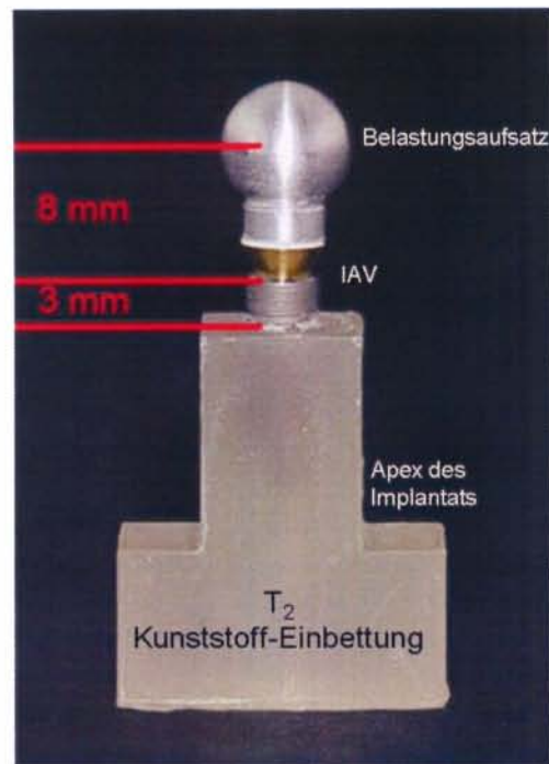
Fig. 17: Directly after releasment from mold. Embedded implant with load attachment (ball cap). DIN 14801 illustration.
