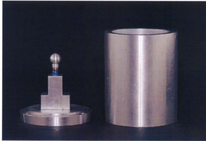
Fig. 10: Embedding form with T1 and implant.
