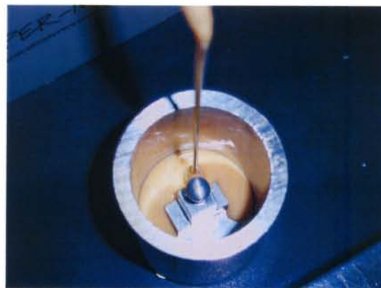
Fig. 11: puring of the silicon into the mold.
