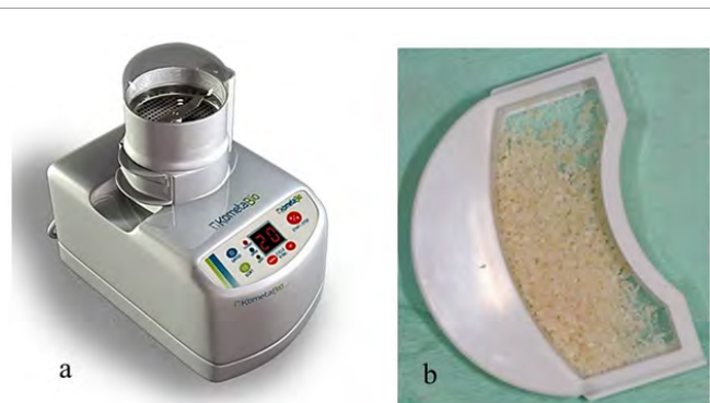
Figure 2: Smart Dentin Grinder and drawer with particulate dentin of 300-1200 µm size ready for cleanser treatment. (a) Smart dentin grinder and sorter. (b) Drawer that collects particulate dentin after grinding and sorting. The size of particles in this drawer are of 300-1200 µm.
